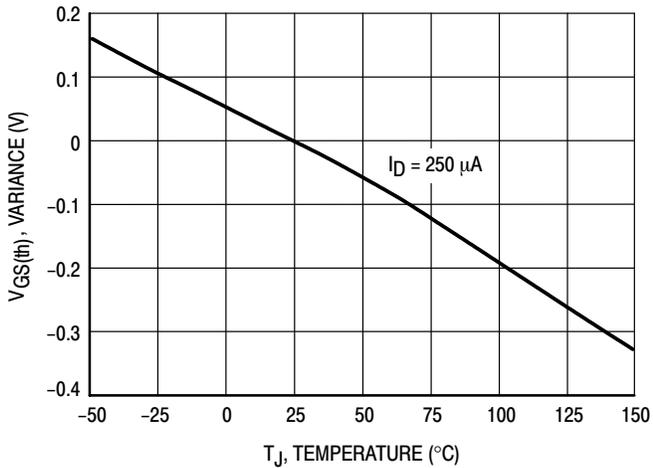
Figure 9. Threshold Voltage
