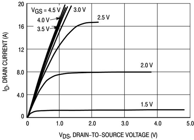
Figure 1. Output Characteristics
