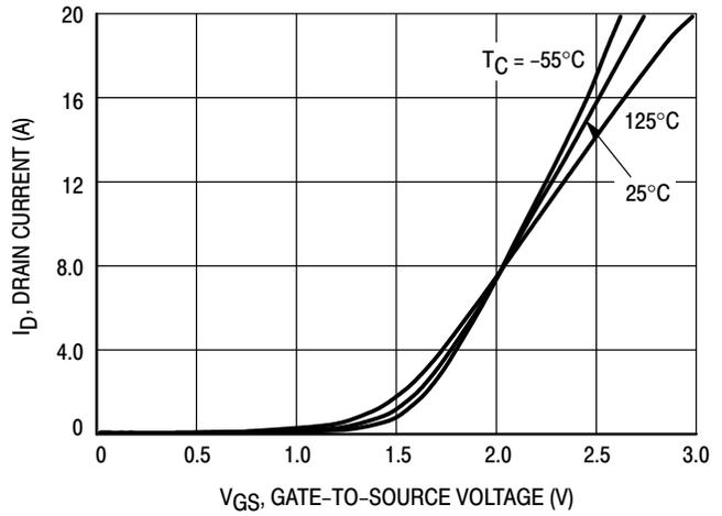
Figure 2. Transfer Characteristics
